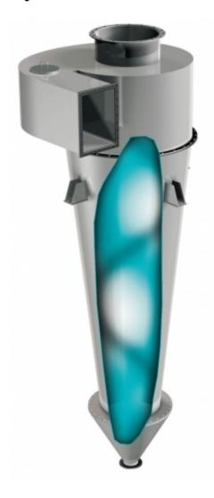
BETH® cyclones are high-efficency separators with an optimised high degree of separation and low head loss. They have proven themselves for many centuries in numerous industrial cases of operation. Depending on the application and kind of dust, they are used as exclusive de-dusting or as a pre-separator.
